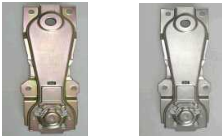
Figure 5. Component with Chromiting (left) and with an additional organic protection coating (SurTec 555, right).
